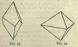
Fig. 33 shows a positive right-handed trigonal trapezohedron.
